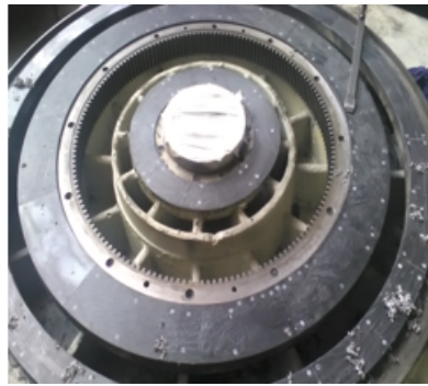
rotational guideways after scraping
