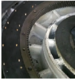
sticking and mechanical clamping of the rotational guideways
