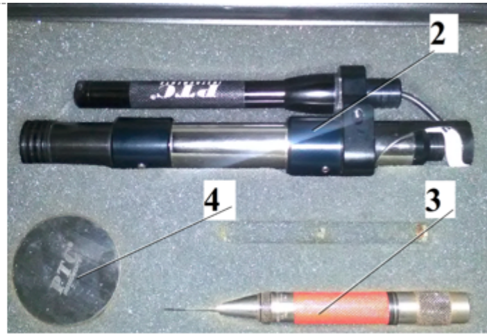
Fig. 10. Measurement of guideways hardness 1 - guideway whose hardness is measured, 2 - fiber optic microscope calibrated, 3 - standard hammer (diamond tip) for performing the hardness test, 4 - standard workpiece
