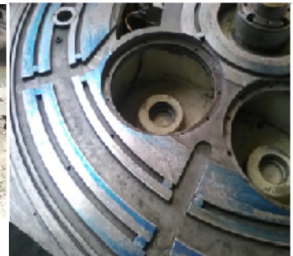
preparation of the rotational guideways surfaces for making the contact spots
